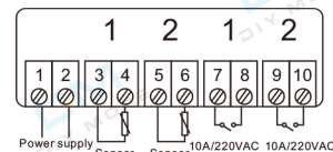
Connection 1: Independent power supply for load
